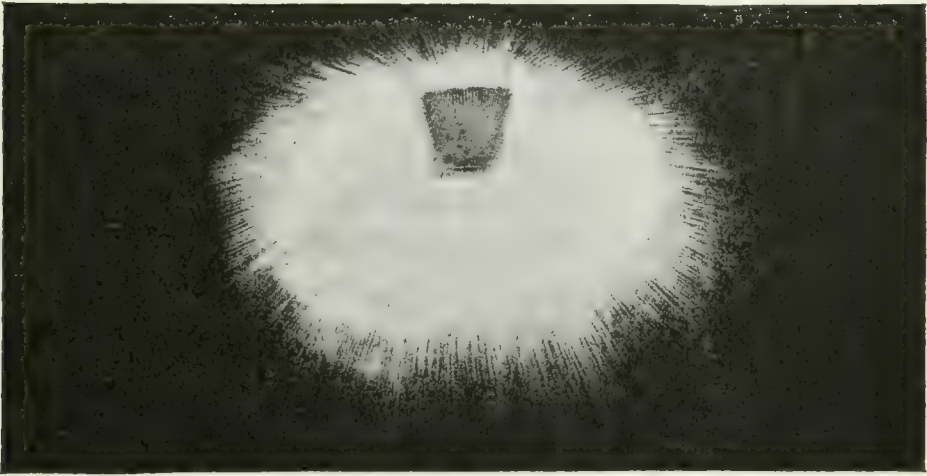
Fig. 75.—Holophane, General Distribution.
